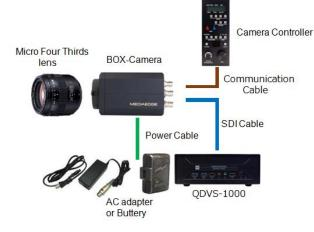
■ Example1: Simple system using metallic cables
