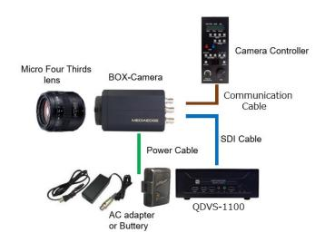
For SDI video output to a nearby QDVS-1100 or other recorders, switchers, servers, and video systems, a direct connection is made from the camera using a coaxial cable. The camera controller is also directly connected to the camera using a communication cable.
